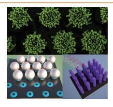
An unique approach to fabricate periodic nanostructures using solution-based synthesis is demonstrated by employing self-developed periodic wettability on a hydrophobic Si substrate in presence of colloidal silica spheres. The feasibility is demonstrated by fabricating circular and ring-shaped patterns of ZnO nanowire ensembles arranged in a hexagonal lattice. Antireflection properties of the fabricated structures are evaluated as a function of feature sizes.
