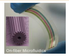
On-fiber microfluidics are introduced as a new platform for the fabrication of disposable microfluidic devices. Well-ordered, perfectly aligned microchannels on polymer fibers are obtained using thermal fiber drawing. Spontenous capillary flow along three-dimensional fiber geometries, switch systems that allow precise control on fluid flow, and a proof of concept colorimetric protein assay are demonstrated.
