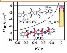
The effect of scaffold alteration on molecular and photovoltaic properties of a series of new D-A-D and their respective D-A systems is elucidated. The D-A-D dyes exhibit significantly improved luminescence and photovoltaic properties compared to those of their D-A counterparts, reaching fluorescence quantum yields of unity in nonpolar solvents and power conversion efficiencies of up to 2.8%.
