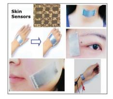
Flexible and wearable strain sensors are assembled by adhering the graphene woven fabrics on polymer/medical tape composite films. The sensors exhibit high sensitivity with notable resistance changes for any tiny deformation and can be used as electronic skin covering human body to detect weak human motions, including hand clenching, phonation, expression change, blink, breath, and pulse.
